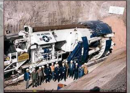
TBM - Tunnel Boring Machine - In the Nevada desert. Photo Department of Energy. The Nevada National Security Site. Perhaps you have heard about tunnels in Area 51 or others.
